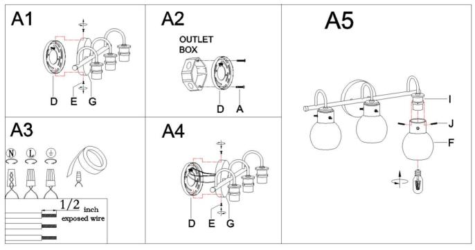
Step A1: Unscrew the studs(E) from the back plate(G) then gently remove the mounting plate (D).Step A2: Secure mounting plate (D) to outlet box with mounting screws (A).Step A3: Make wire connections
