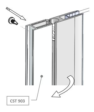
When satisfied with door operation, secure Hinge Post to the Wall Jamb (CST 903) using three 638PHPT Adjustment Screws
