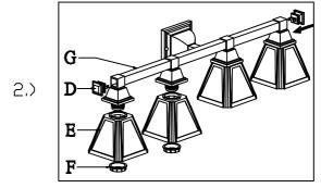
Step 2. Attached the glass(E) on the socket then secure by socket ring(F).
