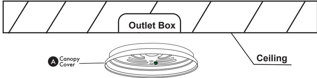
Align canopy cover (A) and outlet screws (B) with outlet box.
