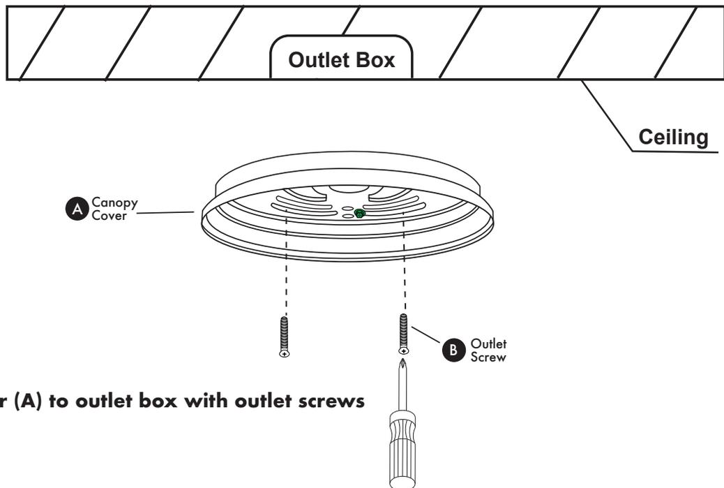
Attach canopy cover (A) to outlet box with outlet screws (B).
