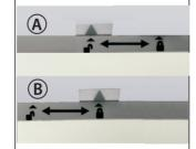
Lift fixture up against bracket. Align the arrow sign  $\blacktriangle$  from bracket to unlock-sign  $\blacksquare$  from fixture. Slide to locked-sign  $\blacksquare$  to lock fixture in place. Remove label.
