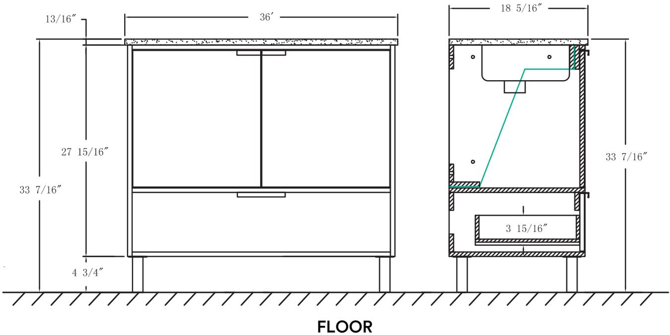
ATTENTION! DIMENSIONS MAY VARY BY UP TO  $\frac{1}{8}$ ". IT IS HIGHLY RECOMMENDED TO PULL ALL DIMENSIONS OF ACTUAL MODEL FOR INSTALLATION AND MEASURING PURPOSES.
