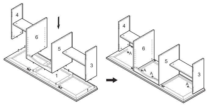
Attach the panel assembly from the previous step to stand top (1) using cam bolts and dowels as guides. Insert cam locks (A) into panels (3,4,5,6) and tighten with a screwdriver. Note that two cam locks will be inserted into each panel.
