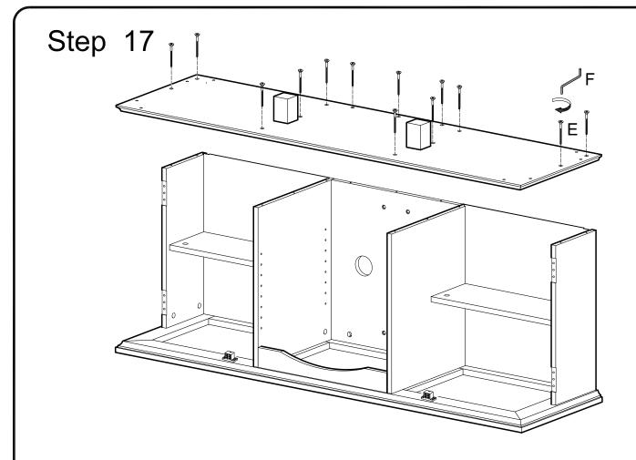
Attach stand base (2) to the stand assembly using bolts (E). Tighten bolts (E) with wrench (F).
