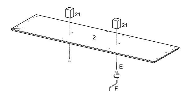
Attach stand supports (21) to stand base (2) using bolts (E). Tighten bolts (E) with wrench (F).
