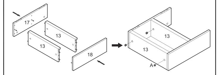
Attach panels (17,18) to the second set of shelves (13) using cam bolts and dowels as guides. Insert cam lock (A) into shelves (13) and tighten with a screwdriver. Note that two cam locks will be inserted into each shelf.
