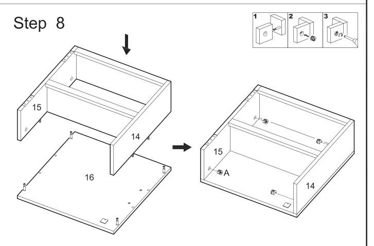
Attach the shelf assembly from the previous step to door (16) using cam bolts and dowels as guides. Insert cam locks (A) into panels (14,15) and tighten with a screwdriver.
