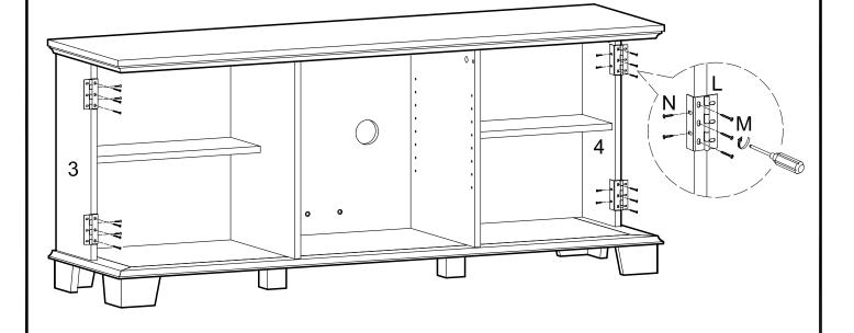
Attach door hinges (L) to panels (3,4) using large screws (M) and small screws (N).
