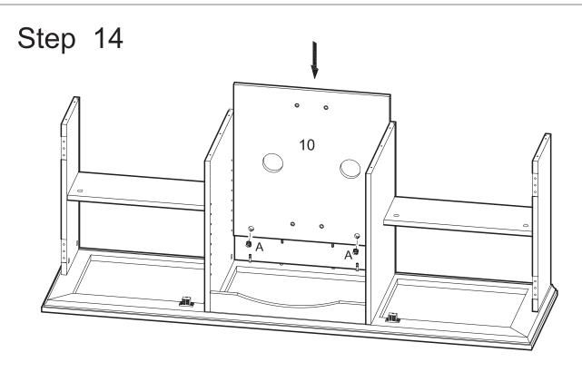
Carefully slide back panel (10) into place along the back of the stand assembly. Use cam bolts and dowels as guides. Insert cam locks (A) into back panel (10) and tighten with a screwdriver.
