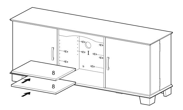
Insert shelf support pins (I) into the stand assembly at desired shelf heights. Carefully slide shelves (8) into place resting on shelf support pins (I).
