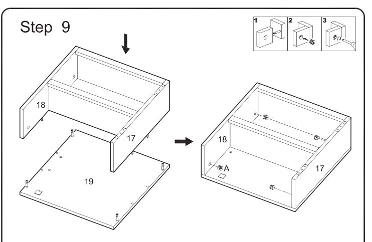
Attach the shelf assembly from Step 7 to door (19) using cam bolts and dowels as guides. Insert cam lock (A) into panels (17,18) and tighten with a screwdriver.
