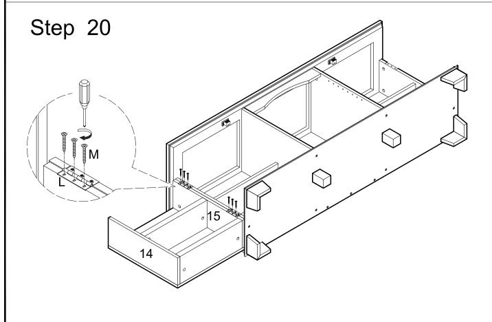
Attach door assembly (14,15) to the stand assembly at door hinges (L) using large screws (M).
