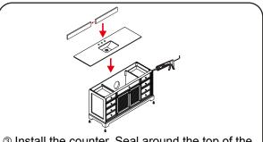
③ Install the counter. Seal around the top of the cabinet with clear silicone sealant. Do not over apply. Allow to dry 24 hours for proper curing.
