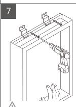
Top mounting brackets must be attached to furring strip/channel or wall strids.
