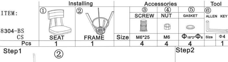
Step 1: Put the bolts(3) through holes of base and swivel.
