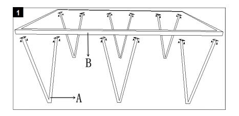
Step 1 Assemble the Leg (A) Top fram (B) together using 24screws(D).
