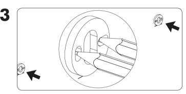
Place mounting plate on the wall and mark position of the holes in the mounting plate.
