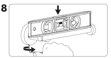
Use the provided allen wrench to adjust the set screw to lock into place with the mounting bracket.
