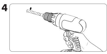
Drill holes in using 1/4" drillbit.
