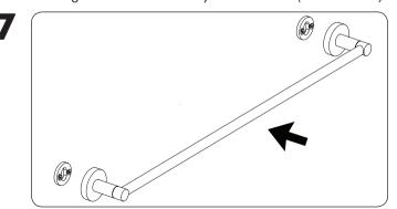
Place towel bar over the mounting plates with the set screw on the bottom.
