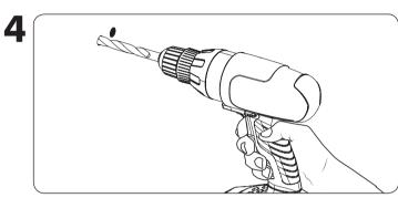
Drill holes in using 1/4" drillbit.
