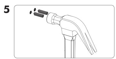
Insert provided anchors if mounting into drywall. Anchors not necessary if mounting into wood studs.
