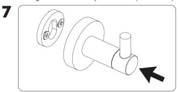
Place the robe hook over the mounting plate with the set screw on the bottom.
