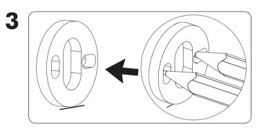
Place mounting plate on the wall and mark position of the holes in the mounting plate.
