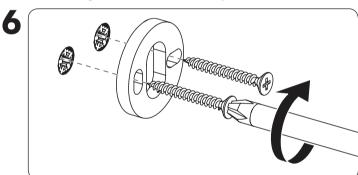
Install the mounting plate with the provided screws.
