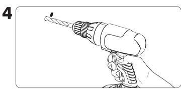
Drill holes in using 1/4" drillbit.
