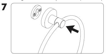
Place item over the mounting plates with the set screw on the bottom.
