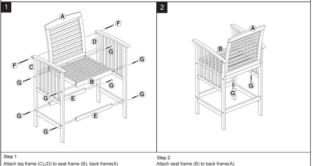
by using screw(G), tighten with allen key(H)
