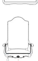
3. Use the Allen Wrench (C) with 4 bolts (D), 4 lock washers (E), 4 Flat Washers (F), attach the ergonomic mechanism to the bottom of the seat.
