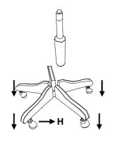
1. Insert the Pneumatic Cylinder into the base, this is a taper fit no mechanical fastening is necessary.
