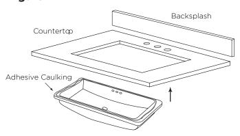
**Step 2:** Locate the 4 metal inserts under the countertop. Attach 4 undermount clips to secure vessel.
