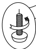
Adjust leveler if needed to level wardrobe on uneven floor.
