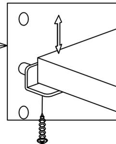
The adjustable shelves are screwed in place to avoid damage during transit. To adjust the shelf height, remove screws then place shelf pins in the desired level.
