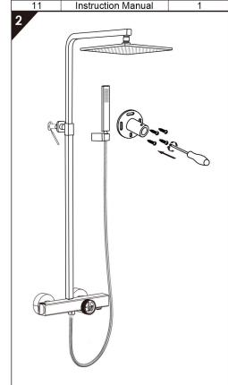
Mark fixing holes, install expansion pipe after wall drilling lock the fixing base on the wall with self-tapping screws.
