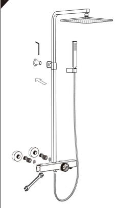
Assemble faucet parts together, install eccentric nipples with decorative covers; Insert gasket and nut and tighten onto eccentric nipples with wrench.
