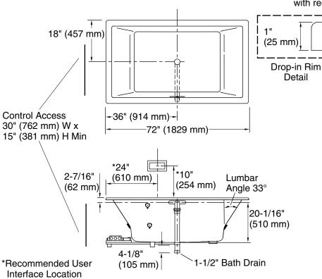
No change in measurements if connected with required drain illustrated. (K-7272)
