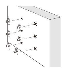
2.Insert the plug (drywall anchors) into the holes that have been drilled.
