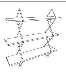
5. Secure the shelf board to the metal rack with small screws.
