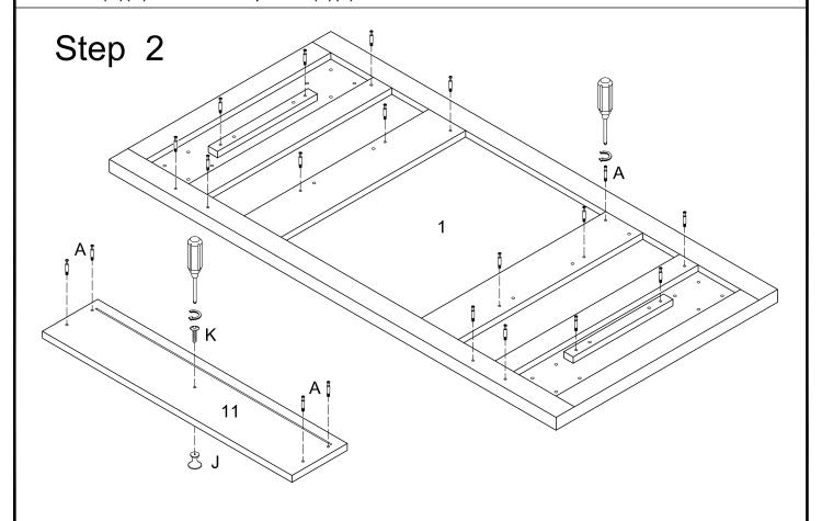
Insert the cam lock (A) into the top panel (1) and drawer front panel (11). Assemble the drawer knob (J) to the drawer front panel (11) and secure it by screw (K).
