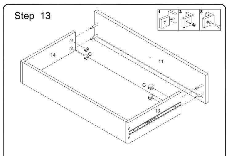
Use cam lock (C) to secure the drawer front panel to the drawer side panels (13)(14).
