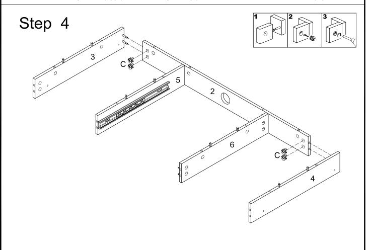
Attach the side panels (3)(4) to the back panel (2) and secure it with the cam lock (C).
