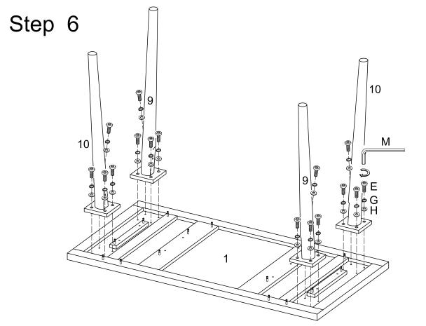
Attach the legs (9)(10) to the top panel (1) and secure it with the washer (H), spring washer (G), bolt (E) and wrench (M). Please do pay attention on the (9)(10).
