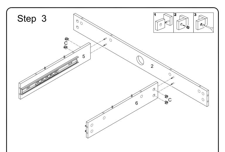
Attach the side panels (5)(6) to the back panel (2) and secure it with the cam lock (C).
