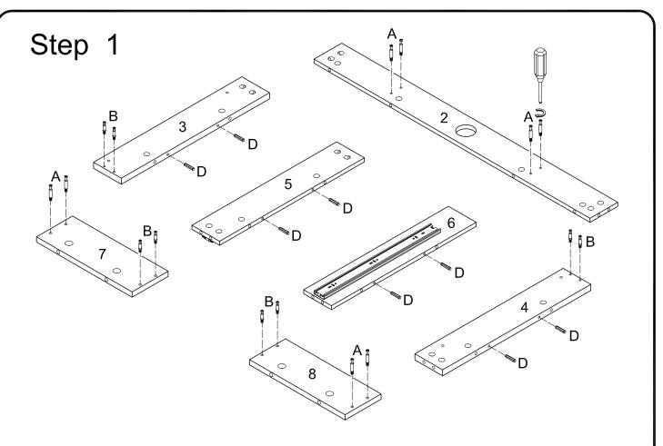
Insert the wooden dowel (D) into the drawer side panels (3)(4)(5)(6). Insert the cambolts (A)(B) into the front panels (7)(8).
