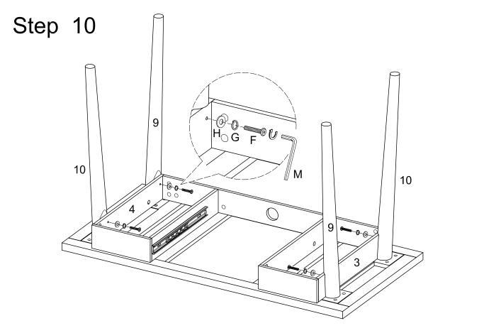
Secure the side panel (3)(4) to the legs (9)(10) by using washer (H), spring washer (G) , bolt (F) and wrench (M).
