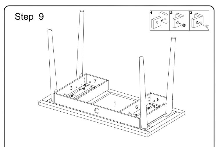
Secure the side panels (3)(6), and front panels (7)(8) to the top panel (1) with cam lock (C).
