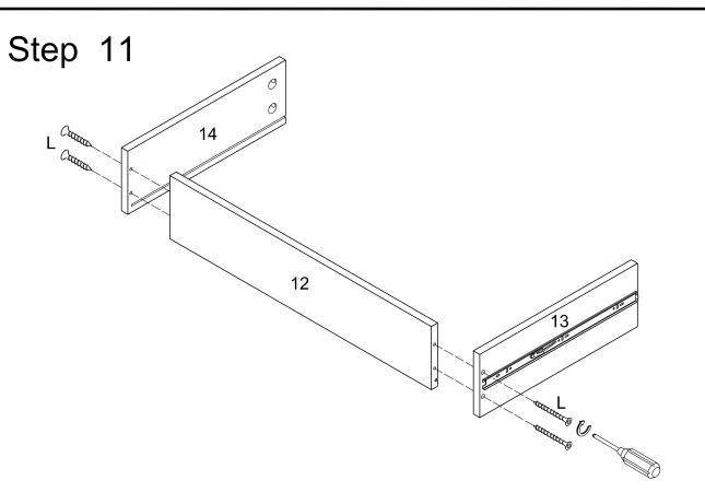
Attach the drawer side panels (13)(14) to the drawer back panel (12) by screw (L).
