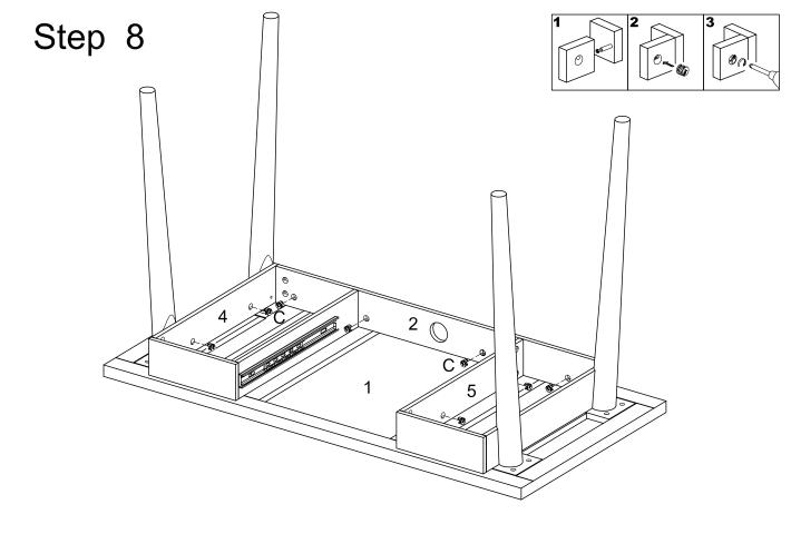
Secure the side panels (4)(5), and back panel (2) to the top panel (1) with cam lock (C).
