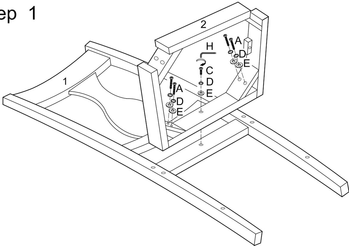
Attach seat frame (2) to chair back (1) using bolt (C), spring washer (D) and washer (E) at the center point and bolts (A), spring washers (D) and washers (E) in the corners. Tighten all bolts (A,C) with wrench (H).
