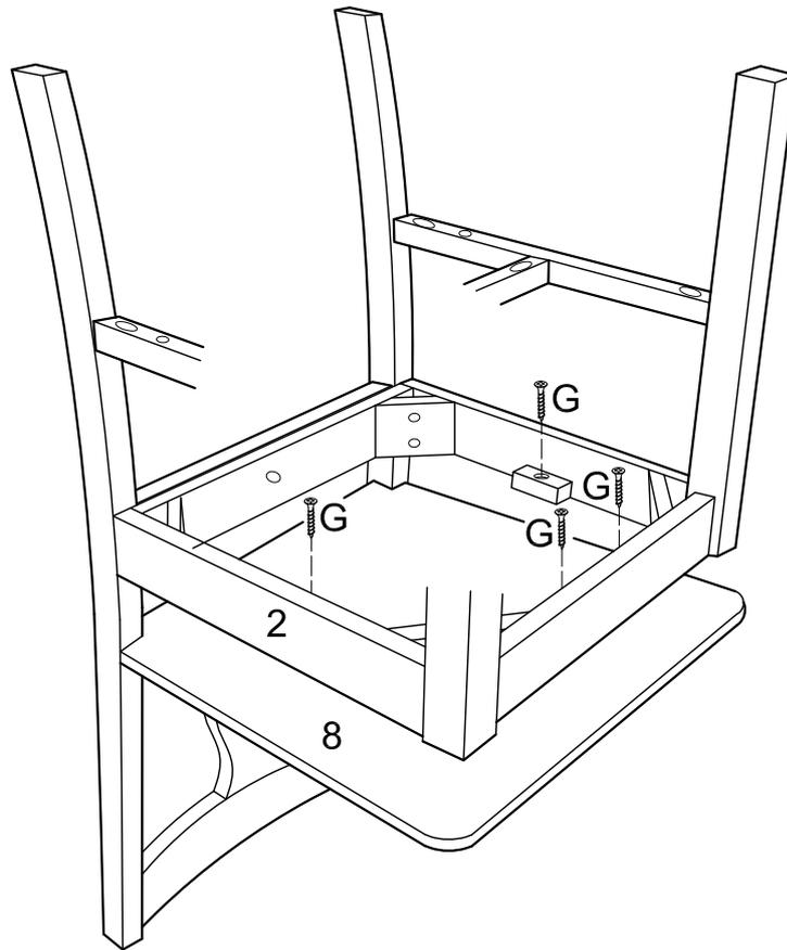
Attach seat (8) to seat frame (2) using screws (G). Tighten screws (G) with a screwdriver.
