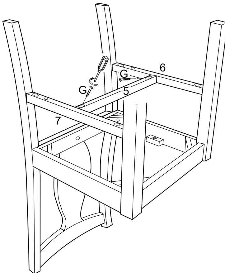
Secure crossbar (5) to crossbars (6,7) using screws (G). Tighten screws (G) with a screwdriver.
