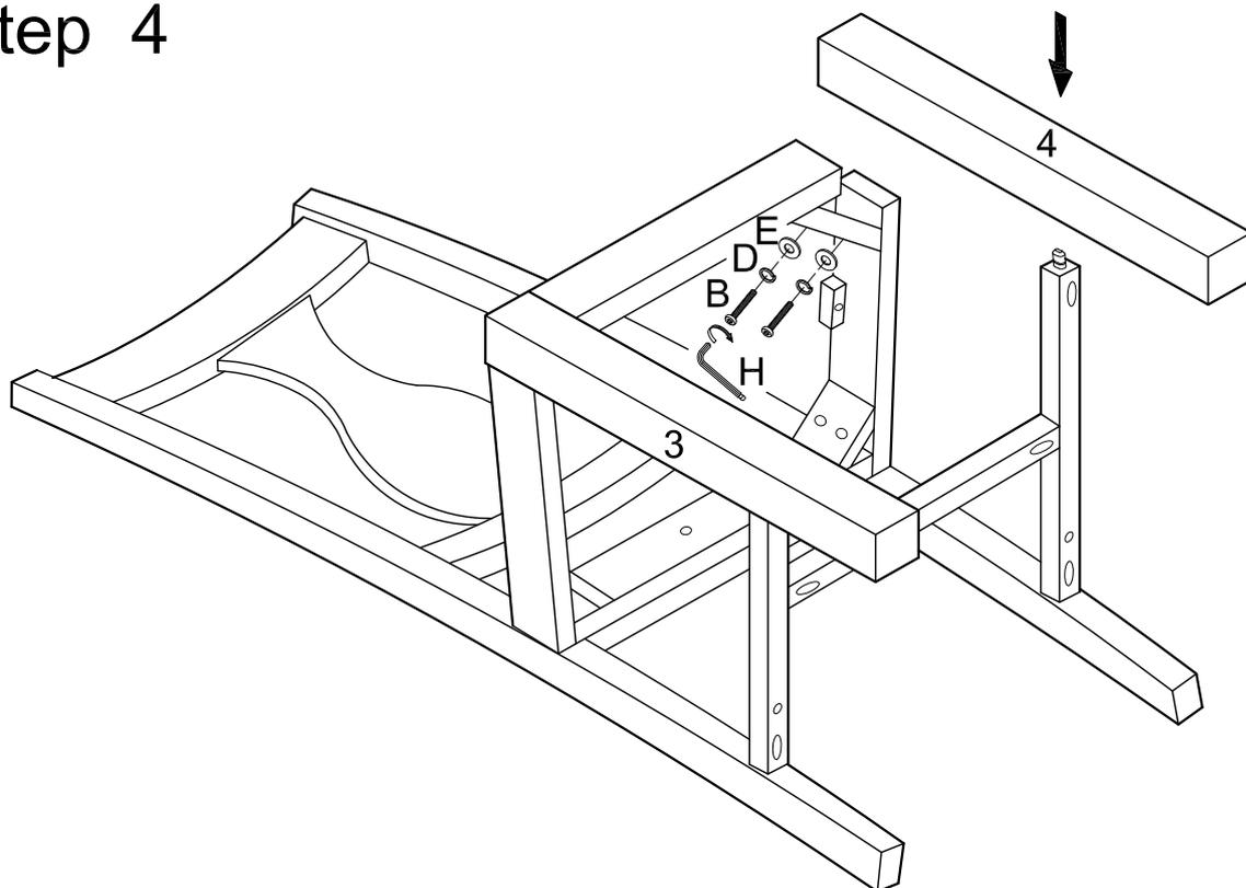
Attach legs (3,4) to the chair assembly using bolts (B), spring washers (D) and washers (E). Tighten all bolts (B) with wrench (H).
