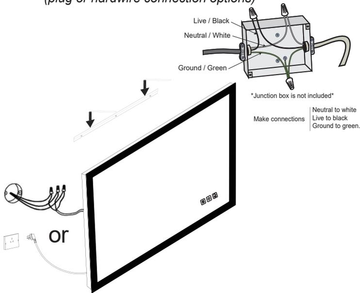
**Warning:** Strip wires to a suitable length. DO NOT connect the hardwire to a plug & socket outlet
