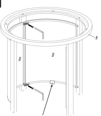
When installing part "D", Please note that the side with this part is facing down.
