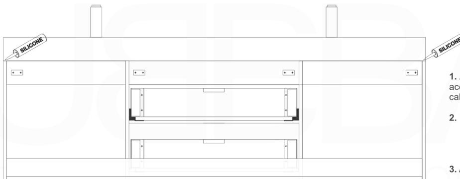
1. Align and level mounting Brackets according to horizontally reinforcement lumber and desired cabinet height.
