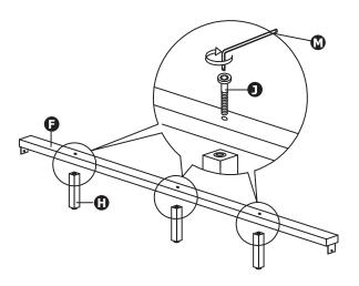
Secure the Footboard Legs (Part E) into the Footboard (Part B). Screw the Center Legs (Part H) into the Center Rail (Part F) using three 40mm Bolts (Part J). Secure the bolts using Small Hex Key (Part M).
