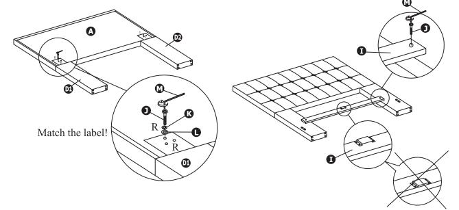
Assemble the Headboard Legs (Part D1 and D2) to the Headboard (Part A) using six 40mm Bolts (Part J), six Spring Washers (Part K) and six Flat Washers (Part L). Use the Small Hex Key (Part M) to secure the bolts. Be sure to use Part D1 for the right side and Part D2 for the left side of the headboard. Next secure the Support Bar (Part I) to the Headboard Legs (Part D) using two 40mm Bolts (Part J). Use the Small Hex Key (Part M) to secure the bolts.
