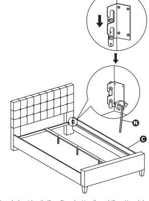
Attach the siderails (Part C) to the Headboard (Part A) and the Footboard (Part B) by hanging the siderails onto the pre-attached bolts on the Headboard and Footboard. Tighten the bolts using Large Hex Key (Part N).
