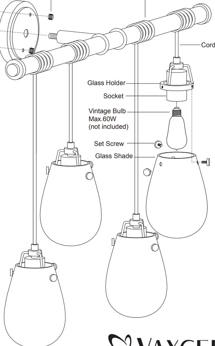
3. Thread two headless screws through the mounting plate, and then secure them with four lock nuts (two on each side of the mounting plate). Adjust the length of the headless screws if necessary.
