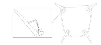
> Please find the hole which marked at bottom. Put legs at the right location.> Fix the screws by wrench on the hole one by one. Total 3 screws for one leg.> Fix other legs as the same way as first one
