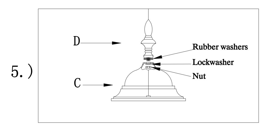
Step.5: Install the finial(D) into the cover(C), using the nuts
