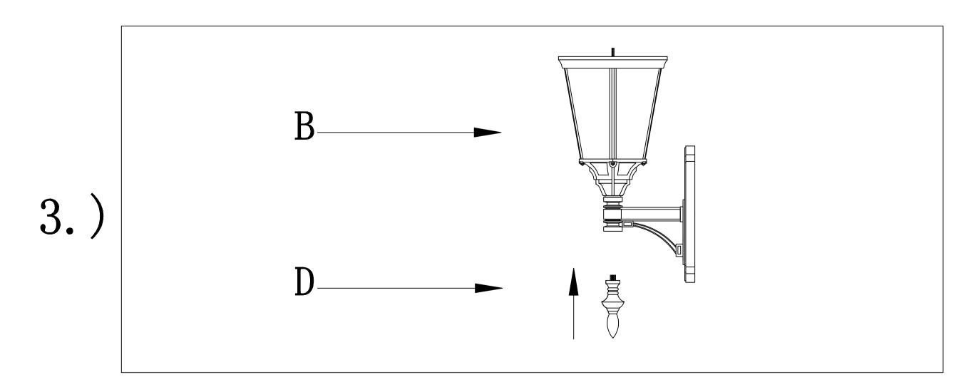
Step.3: Install the finial(D) into the fixture(B)
