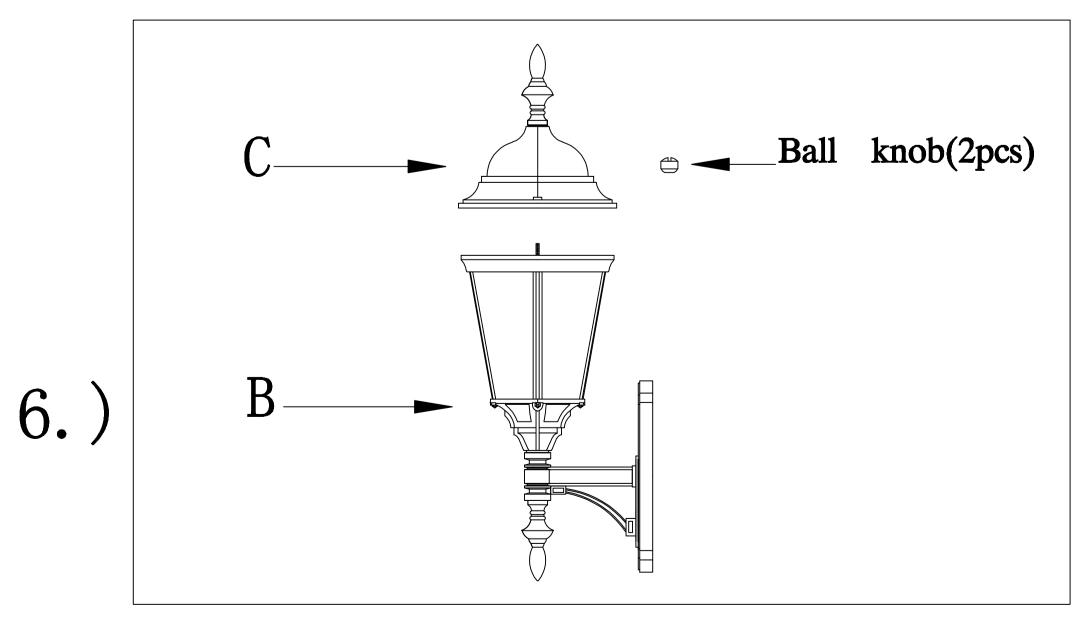
Step.6: Install cover(C) to fixture, using ball knobs.
