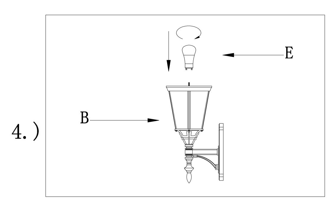
Step.4: Install GU24 LED bulb(E)
