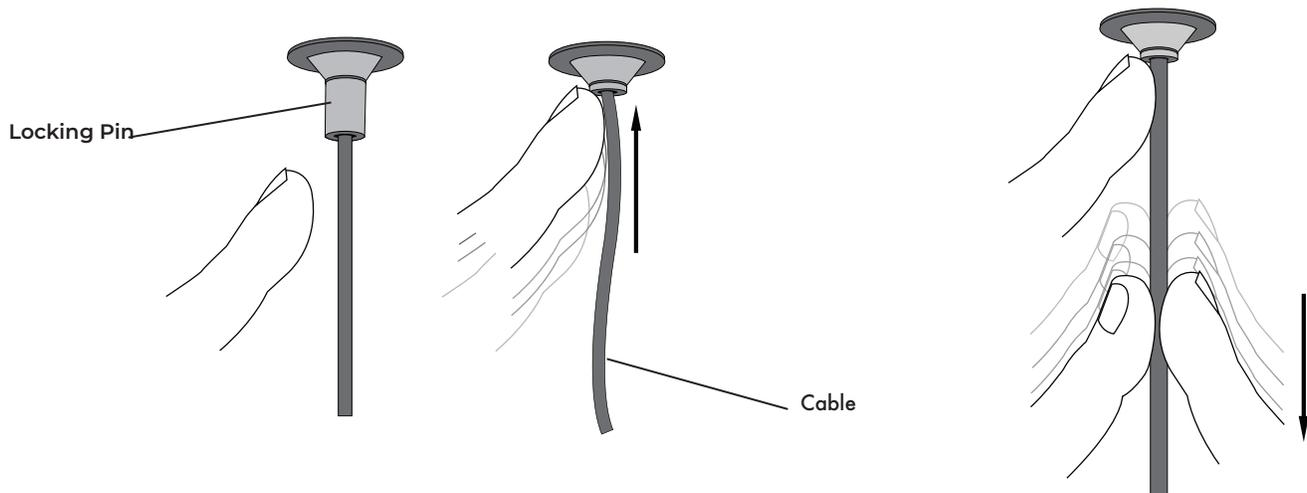
**The length of the cable is adjustable. To determine the proper length of the fixture, hold the fixture canopy up against the outlet box in the ceiling to adjust the cable.**
