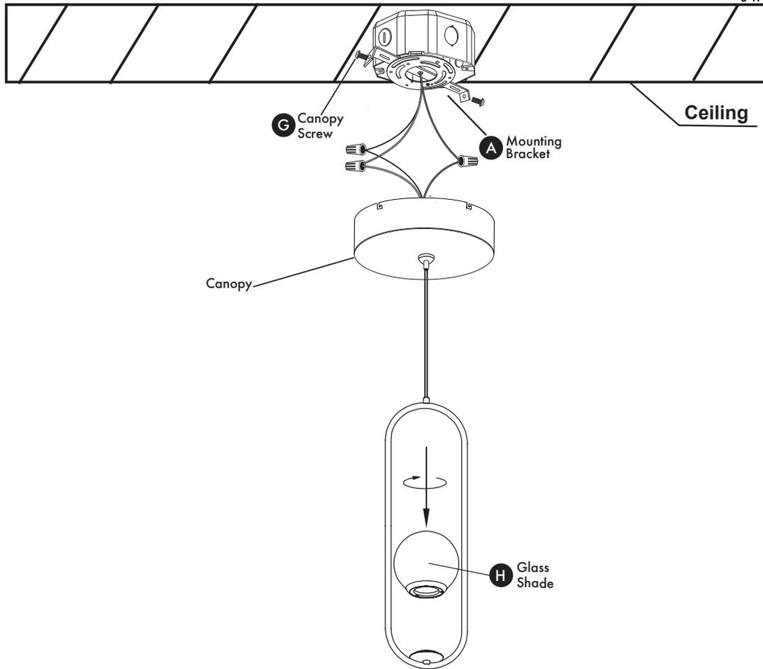
**Attach canopy to mounting bracket (A). Twist canopy to lock fixture in place. Secure canopy with canopy screws (G). Attach glass shades (H).**
