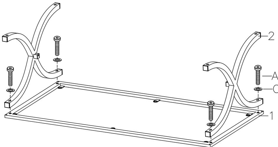
Attach side panel (2) to top frame (1) using bolts (A) and flat washer (C) as shown.
