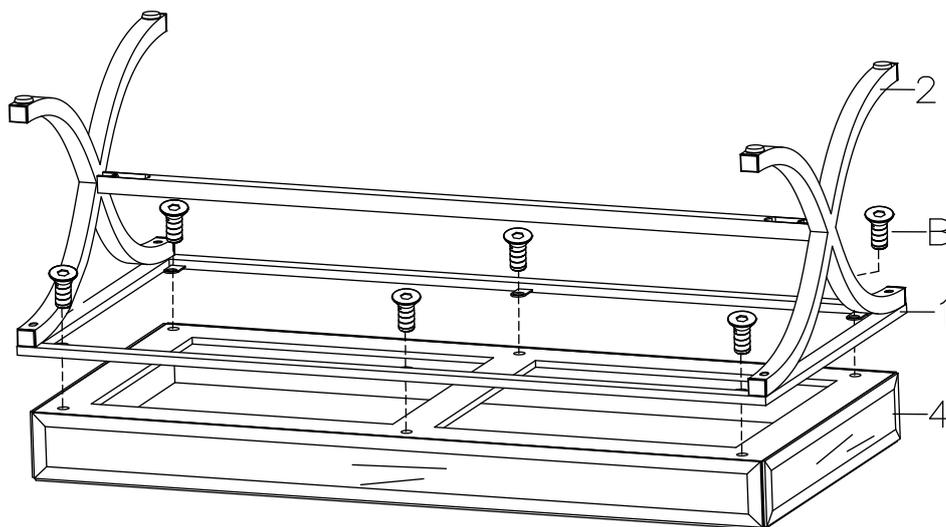
Attach the assembled parts to mirrored top (4) using bolts (B) again. Tighten all bolts and carefully turn the assembled unit upright.
