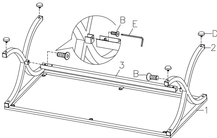
Attach stretcher (3) to side panel (2) using bolts (B) with wrench (E). Then, attach leveler (D) to the bottom of side panel (2) as shown.
