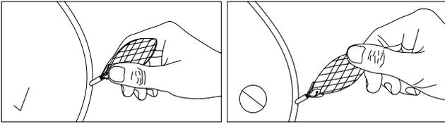
**Hold the crystals carefully by the metal base to prevent the crystals from cracking or breaking.**
