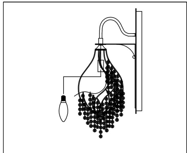
**Step. 4:** Install max 60 watt candelabra bulb (not included) into socket.
