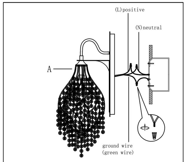
**Step. 2:** Carefully unwrap fixture. Wire fixture to wires in outlet box. Copper/green wire is for Ground.
