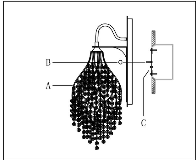
**Step. 3:** Attach fixture to mounting bracket (C) and tighten with Ball nut (B).
