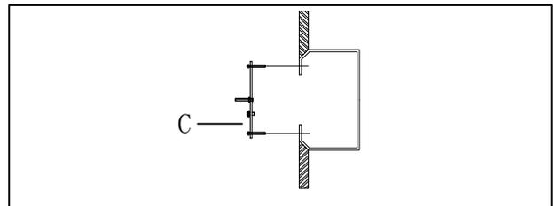
**Step. 1:** Install mounting bracket (C) to outlet box.
