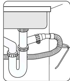
Figure 12: Secure the drain hose to the sink wall using cable ties or other fastening materials. Otherwise, the drain hose may bend at the end causing a drainage problem or excessive supply of water.
