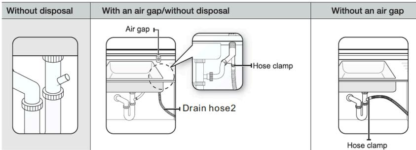
3. Check the size of the sink's drain hose connector (21 mm (0.83 inches)- as shown in Figure 11 on the next page). If the end of the drain hose does not fit onto the drain hose connector of the sink, use an adapter purchasable at a plumbing/hardware supply store.
