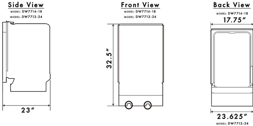
The water supply line, power cable, and drain hose should go through the space behind the dishwasher. The power cable runs in channels under the dishwasher to connections in the front.
