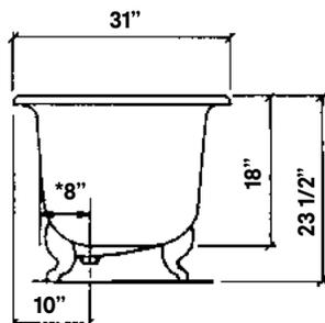
\*8" C.C. waste/overflow to drain
