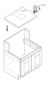
Step 10: Place the sink over the plywood. Check that the drain and faucet-line cut-outs line-up correctly. Confirm that the sink is leveled and adjust if not.
