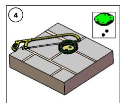
Remove the cover and outlet plugs from the rough-in part. Cut off the excess plastic portion of the roughin part.
