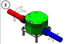
Connect the hot and cold water supplies to the rough-in part. Use thread adapters where needed. Check for any leaks.
