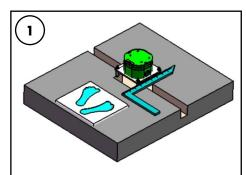
Place the rough-in part in the desired position. Mark and drill (4) holes.
