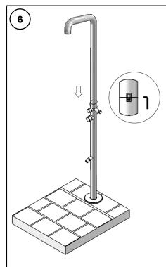
Insert the upper half of the shower into the lower half while connecting the flexible hose. Align the rectangle on the back side of the shower and secure the set screw.
