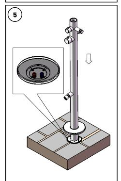
Install the lower half of the shower onto the rough-in part. Secure into place with (4) screws. Carefully lower the base plate cover onto the finished floor.
