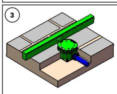
Ensure the rough-in part is level and aligned. Secure by tightening the (4) expansion bolts. Make sure the rough-in part does not protrude from the finished floor by more than 1 inch (25 mm).
