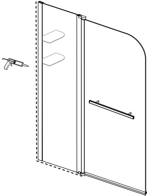
The sealant should be applied to the outside edge.
