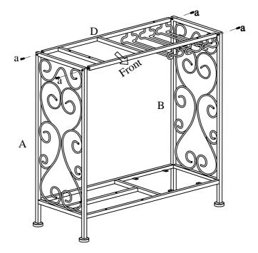
Assemble Top Frame (D) to Side Frames (A&B) using Bolts (a). Please do not tighten Bolts (a) until step 5.
