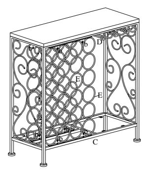
Assemble Wine Holders (E) to Top Frame (D) and Bottom Frame (C) using Bolts (b). Please do not tighten Bolts (b) until step 5.
