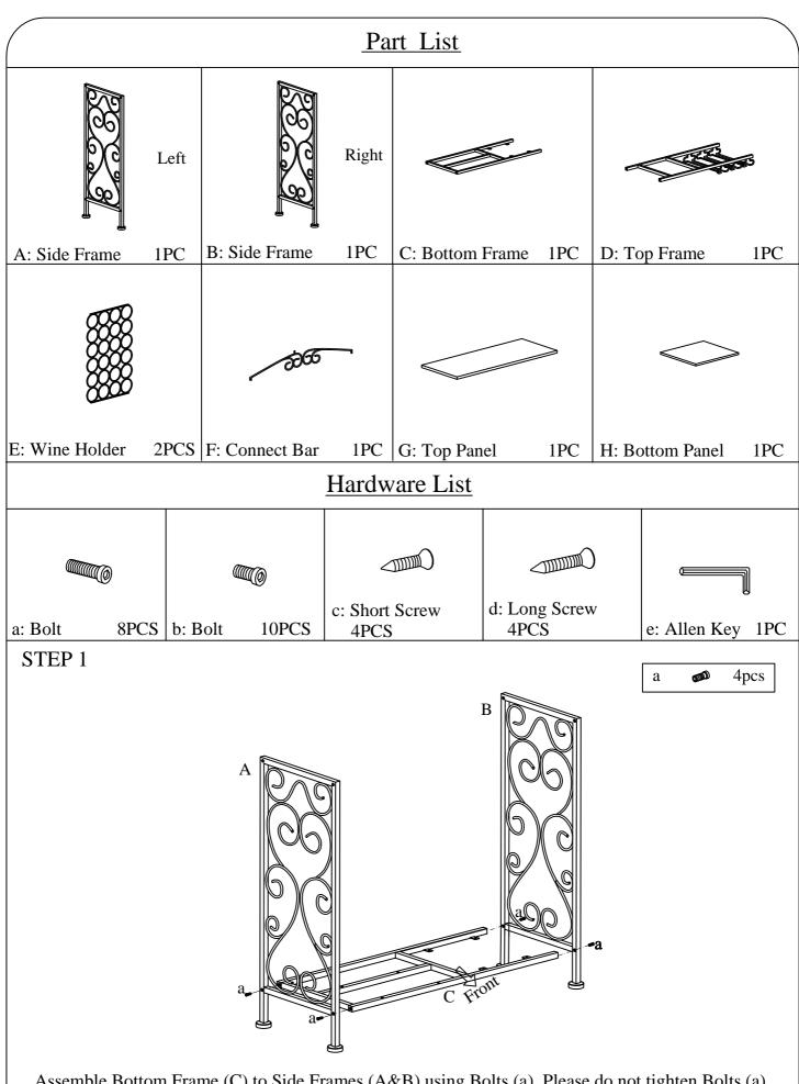
Assemble Bottom Frame (C) to Side Frames (A&B) using Bolts (a). Please do not tighten Bolts (a) until step 5.
