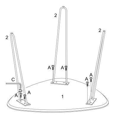
Use wrench (C), bolt (A) to secure the metal leg (2) to the table top (1).
