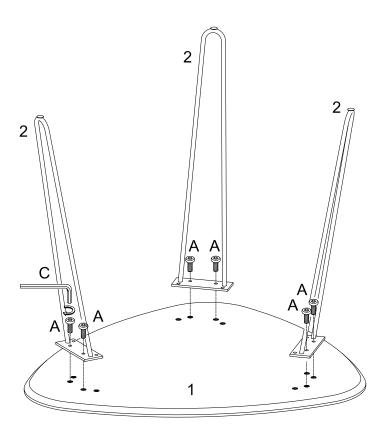
Use wrench (C), bolt (A) to secure the metal leg (2) to the table top (1).
