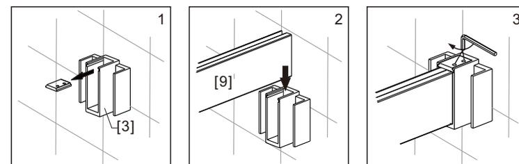
4. Remove the covers of the Wall Connectors[3], stick the two ends of the Top Horizontal Rail[9] in the Wall Connectors[3]. Recover and fasten the covers with Allen Key.
