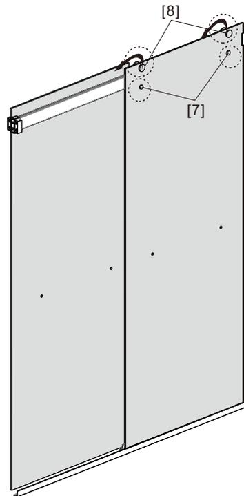
7. Install the Top Rollers[8] into the two pre-drilled holes of the Door Panel[16]. Place the bottom of Door Panel[16] into the gap between the Door Guide[10] and Bottom Horizontal Rail[13], and insert the top of Door Panel[16] into the slot of Top Horizontal Rail[8]. Install the Anti-collision Component[7] into the hole of Door Panel[16],lock and fasten it.
