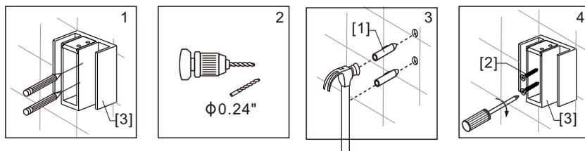
3. Measure a distance of 53.6" from the bathtub to Wall Connectors[3], and mark the holes' position for Wall Connectors[3]. The left and right Wall Connectors[3] must align with each other.
