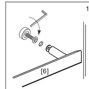
8. Install the Handle Set[6] onto the Door Panels[5&16], lock and fasten them with Allen Key. Please see Fig 1 for details.
