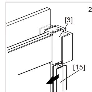
Press the Door Side Gasket[15] onto the vertical edges of the Door Panels[5&16]. Please see Fig 2 for details.
