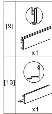
2. You need to cut the Top Horizontal Rail[9] at one end to be length of  $W-0.4$ ", and the length to cut off will be L:
