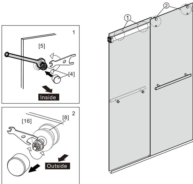
9. If there is a seam when the door is closed like the picture in the right, use Wrench to adjust the Top Wheel [4] or the Top Roller [8] till there is no seam any more.
