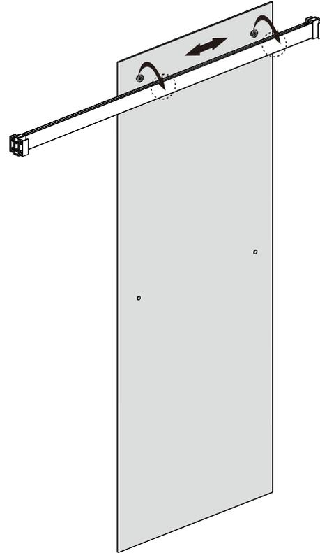
5. Install the Top Wheels[4] through the pre-drilled holes in Door Panel[5]. Stick the Top Wheels[4] in the openings of the Top Horizontal Rail[9].
