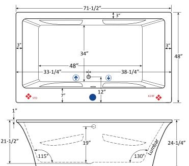
Specifications and features are subject to change without notice and are + .25". All final measurements should be taken from tub on site. HydroMassage Products LLC • 303-341-1845 • Fax: 303-341-1850 • www.hydromassageproducts.com
