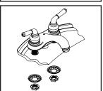
(2) Place the faucet in position on the sink. Slide the crowfoot washer through shank from underneath of the mounting surface and tighten with small plastic locknut with the help of 1-3/32" socket.
