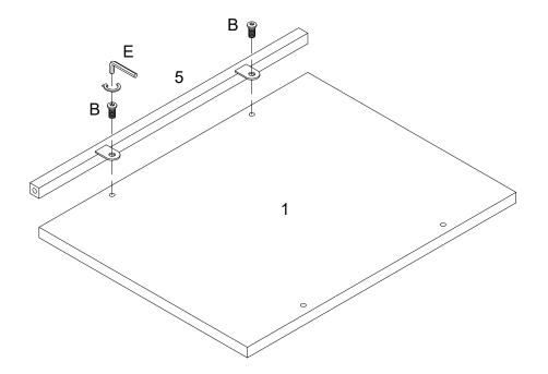
Attach part (5) to part (1) using bolt (B) with hex key (E).
