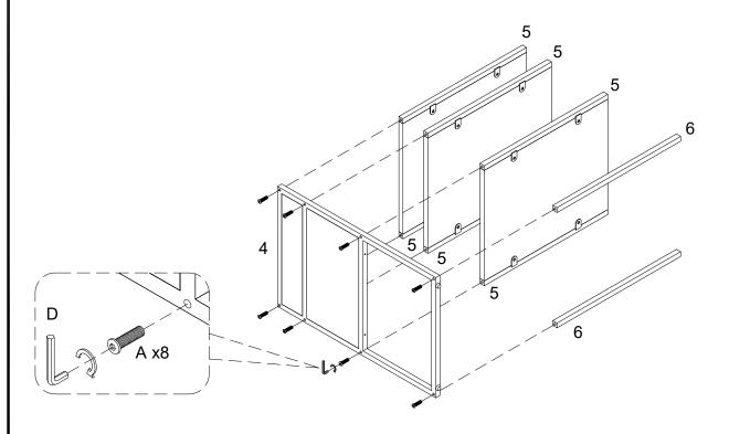
Attach part (4) to part (5,6) using bolt (A) with hex key (D).
