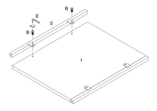
Attach part (5) to part (1) using bolt (B) with hex key (E).
