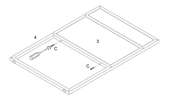
Attach part (4) to part (3) using screw (C) with screwdriver.
