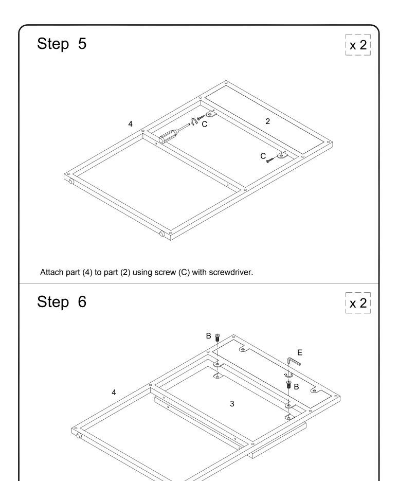
Attach part (4) to part (3) using bolt (B) with hex key (E).
