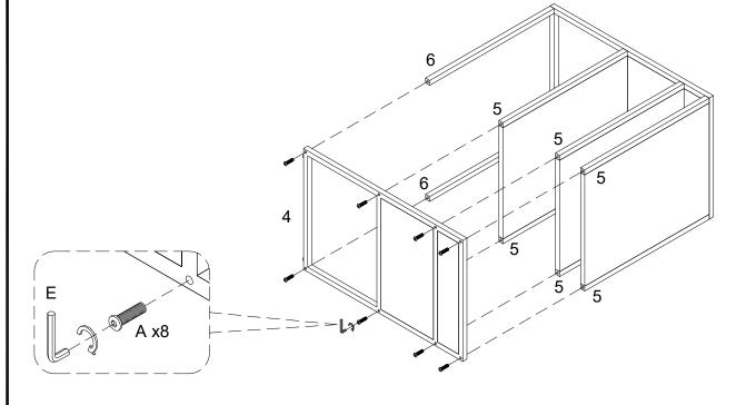
Attach part (4) to part (5,6) using bolt (A) with hex key (D).
