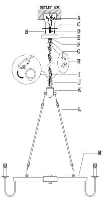
Step A1: Adjust the arms (M) to the proper position.
