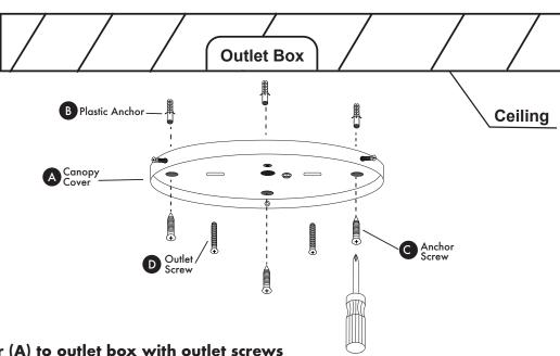
Attach canopy cover (A) to outlet box with outlet screws (D). Screw anchor screws (C) into plastic anchors (B) to secure canopy cover (A).
