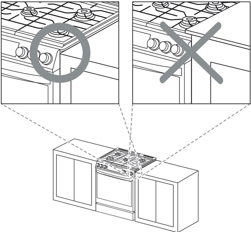
3. Using 2 or more people, gently move range into its final installation location and insert the rear range foot into the slot of the anti-tip bracket, being careful not to damage countertops, floor, or appliance.
