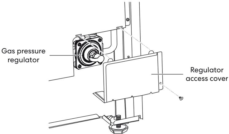
4. If present, remove the plastic dust cover on the regulator plug.
