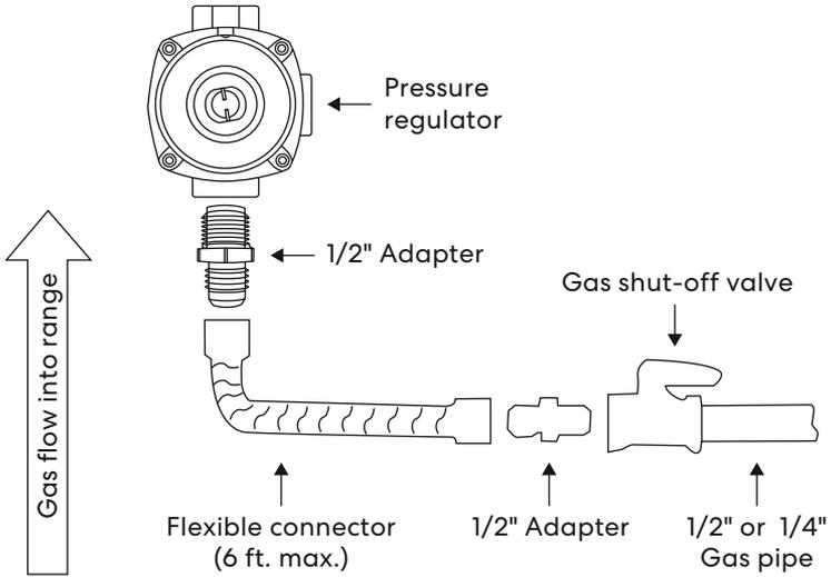
1. Turn manual shut-off valve to the closed position.
