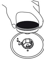
2. Remove the existing gas orifices with a 9/32" (7 mm) nut driver.
