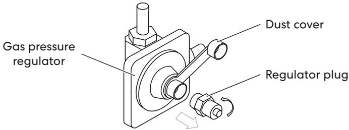
**6. Orient the regulator plug for the fuel type being used.**
