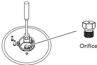
3. Replace the orifices with the correct fuel type orifices. Gas orifices are stamped with a size number. Refer to the orifice chart earlier for correct Natural gas and LP gas orifice sizes and ratings for proper placement.
