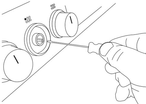
**IMPORTANT:** Adjustments must be made with all other burners in operation on the highest setting. This prevents the flames from being set too low, resulting in the flame being extinguished when other burners are turned on.
