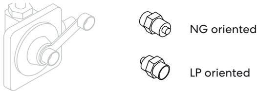
**7. Screw and tighten the regulator plug back into the gas pressure regulator with an adjustable wrench, and replace the plastic dust cover if present.**
