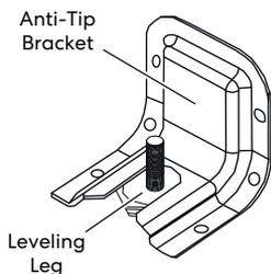
Making sure the anti-tip bracket is installed:
