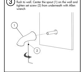
Slide spout (1) over exposed stub out pipe until
