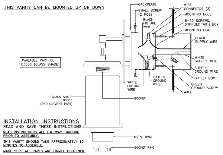
CAUTION: TO AVOID POSSIBLE ELECTRIC SHOCK, MAKE SURE THE ELECTRICITY IS SHUT OFF AT THE MAIN PANEL. IF YOU ARE REPLACING AN EXISTING FIXTURE, FIRST TURN THE FIXTURE OFF. NEXT, TURN THE WALL SWITCH OFF. FINALLY, GO TO THE MAIN FUSE OR BREAKER BOX IN YOUR HOME. TURN THE FUSE OR BREAKER TO THE OFF POSITION. SOME TYPES OF FUSES MUST BE UNSCREWED TO SHUT OFF THE POWER.
