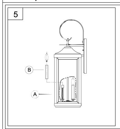
5. Attach candle covers (B) to fixture (A). Screw lamps (not included) into fixture sockets. Use 60-watt MAX incandescent candelabra base lamp, SBCFL or SBLED.
