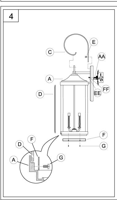
4. Put one end of the scroll (C) through the fixture (A), then attach other end to the canopy using the cylinder screw (E) to secure tightly. Install fixture (A) to screw (AA) using ball nut (EE) and waterproof o-ring (FF).
