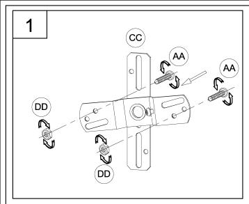
1. Screw screw (AA) onto Swivel mounting strap (CC) and use hex nut (DD) to secure it tight.
