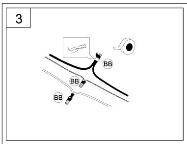
3. Strip 3/8" of insulation from the electrical wire ends. Using wire nuts (BB), connect white fixture wire to the white supply wire from the outlet box; connect the black fixture wire to the black supply wire.
