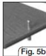
TRIM MOULDED SCREEN RIB 3/8" FROM EDGE
