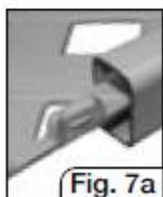
SLIDE C-CHANNEL OVER TABS OR PINS
